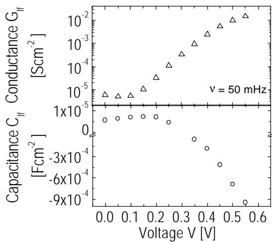
*Figure 2: The low-frequency conductance  $G_{lf}$  of the solid-state DSSC increases exponentially under forward bias  $V$  whereas  $C_{lf}$  becomes negative for voltages  $V > 0.3$  V.*
