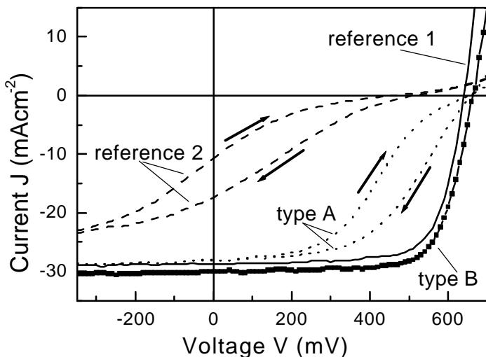
Figure 1: Current-voltage characteristics of illuminated samples. The arrows show the direction of applied voltage bias for the devices that exhibit the IV hysteresis (reference 2 and type A). The IV curves of CdS and type B devices have almost the same values in both directions of measurement.
