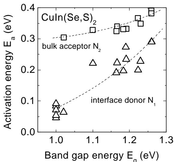
Figure 1: The activation energies of the interface donor  $N_1$  and the bulk acceptor  $N_2$  increase with increasing band gap energy, if CulnSe<sub>2</sub> is alloyed with S. Dashed lines are guides to the eyes.
