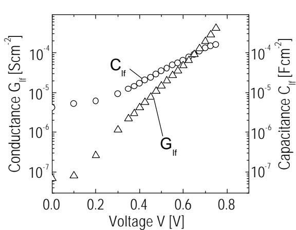
*Figure 1: The exponential increase of the low-frequency capacitance  $C_{lf}$  and of the conductance  $G_{lf}$  is explained by the injection and diffusion of electrons in the  $TiO_2$ .*
