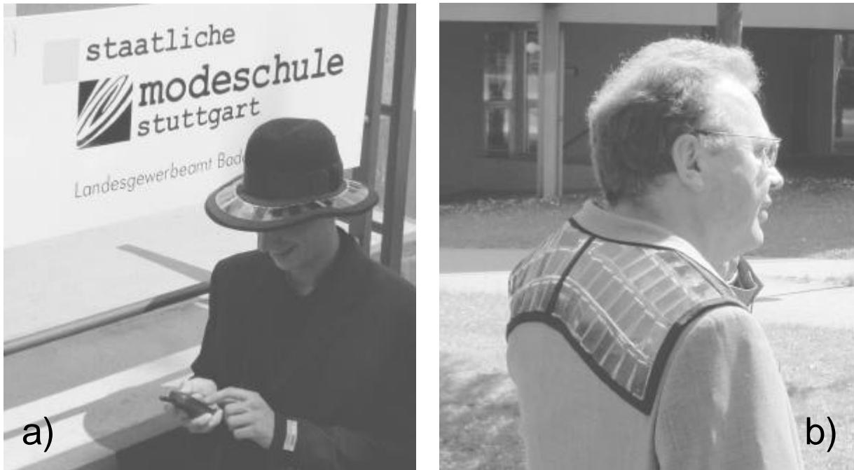
*Figure 1: The figures demonstrate the successful construction of the solar hat (figure 1a) and jacket called Jack I (figure 1b) and emphasize the fact, that the integration of photovoltaics onto clothing meets modern fashion design. Monocrystalline silicon is the base material of the solar cells that supply energetically mobile communication electronics such as cellular phones, personal digital assistants (PDAs), MP3 players, radios and world receivers.*
