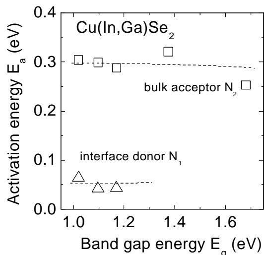
Figure 2: The activation energies of  $N_1$  and  $N_2$  remain constant, if the band gap of CulnSe<sub>2</sub> is increased by alloying with Ga.
