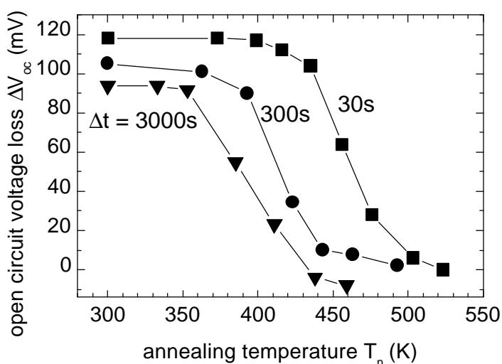
Figure 1 : The decrease of the open circuit voltage loss  $\Delta V_{oc}$  towards zero with stepwise increased annealing temperature  $T_n$  shows that, after sufficient annealing, the devices completely recover from the radiation damage. The time steps  $Dt$  for the isochronal annealing experiments in air are  $Dt = 3000$  s (triangles), 300 s (circles), and 30 s (squares).
