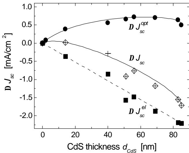
Figure 1: Optical gain  $\Delta J_{sc}^{opt}$  (circles), electronic loss  $\Delta J_{sc}^{el}$  (squares), and the total current density change  $\Delta J_{sc}$  (crossed diamonds). The upper two datasets are connected with spline curves as guides to the eye, the electronic loss follows a linear fit. Optical gain and electronic loss almost compensate each other for CdS thicknesses between  $d_{CdS} \gg 0$  and 40 nm.
