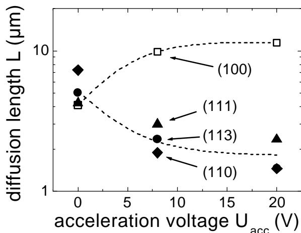
*Figure 1: Influence of ion energy on the minority carrier diffusion length  $L$  of films deposited at  $T_{\text{dep}} = 650^\circ\text{C}$ . In the case of (100)-oriented films an increase of the acceleration voltage from 0 V to 8 V results in an increase of  $L$  by more than a factor of two. However, for non-(100)-oriented films the minority carrier diffusion length decreases with rising ion energy.*
