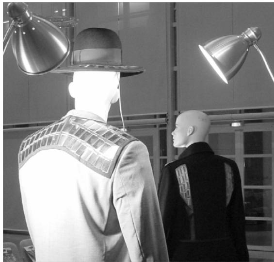
*Figure 1: Demonstration of garment integrated photovoltaics. These first prototypes use rigid high-performance crystalline silicon cells, and one single charge controller for all strings connected in parallel.*
